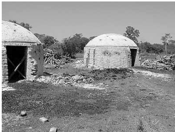
Figure 7 Improved traditional charcoal production: a Brazilian-type brick kiln in Cuba. Source Stassen (2002)
