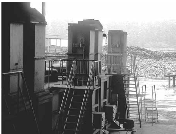
Figure 8 Industrial charcoal retort in the Netherlands, Source Stassen (2002)
